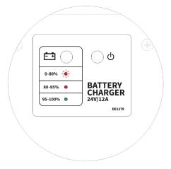
FIGURE 24: Battery Charger LED Display
