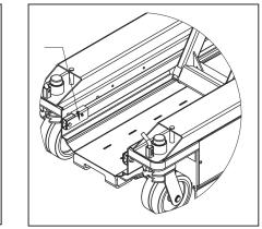
FIGURE 2: Maintenance Lock Pin Storage
